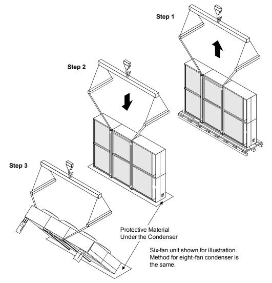
Figure 15 Attaching sling to a 6-fan or 8-fan unit for moving
